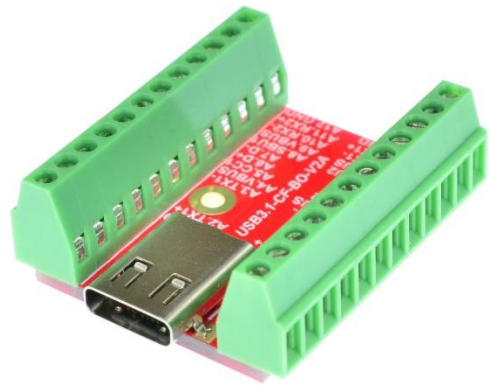
Figure 4: USB3.1-CF-BO-V2A with terminal blocks
