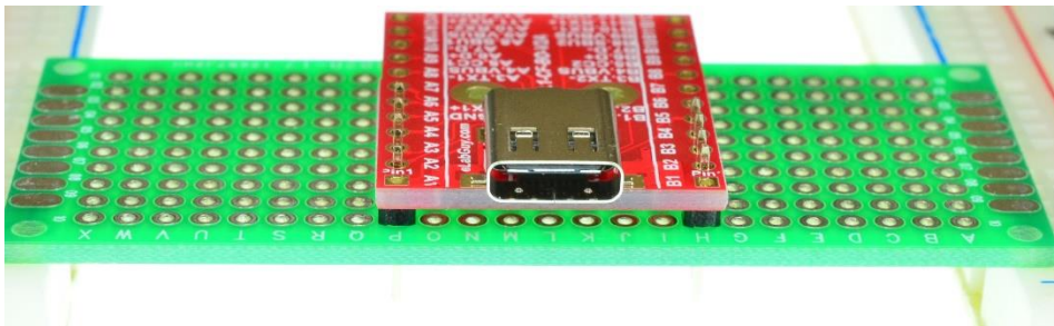
Figure 5: Solid Mounting on prototype PCB
